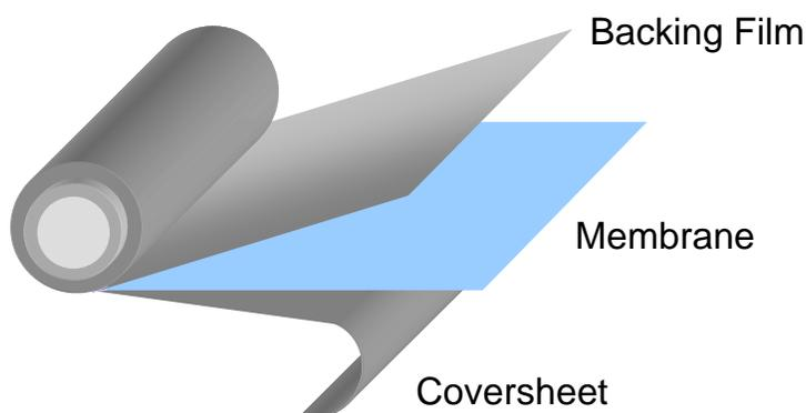
The 3.0-mil backing film facilitates transporting the membrane into automated MEA fabrication processes, while the 0.92-mil coversheet protects the membrane from exposure to the environment during intermediate handling and processing. In addition, the coversheet (in combination with the backing film) eliminates rapid changes in the membrane's moisture content, and stabilizes the dimensions of the membrane as it is removed from the roll.
